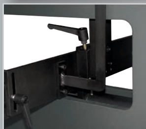
Limit stop system in Y direction Mobile, 2 guide shafts in press body.
