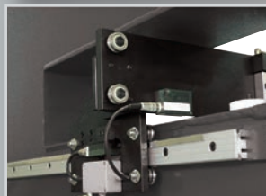
Path measurement of X and Y travel
