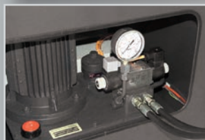
Dual-circuit hydraulic unit in cabinet base
