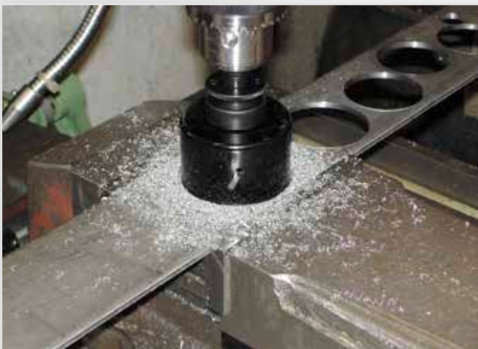
Also steel/stainless steel up to approx. 3 mm, can be worked easily (for frequent use, we recommend our TCT Hole Saws).
