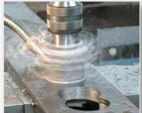
Drilling in flat steel
