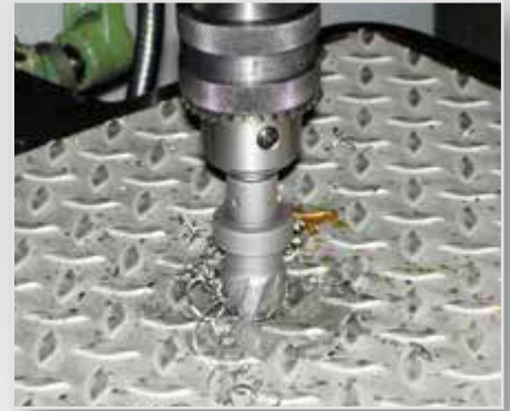
Drilling structured sheet metals
