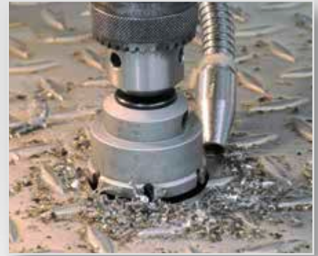
Drilling in checker sheet
