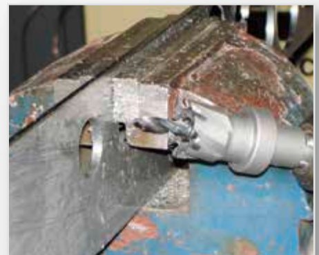
Free-hand drilling up to Ø 30 mm
