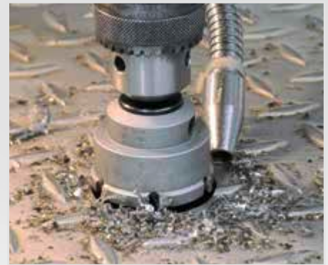
Drilling in checker sheet
