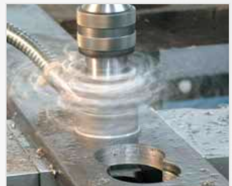
Drilling in flat steel
