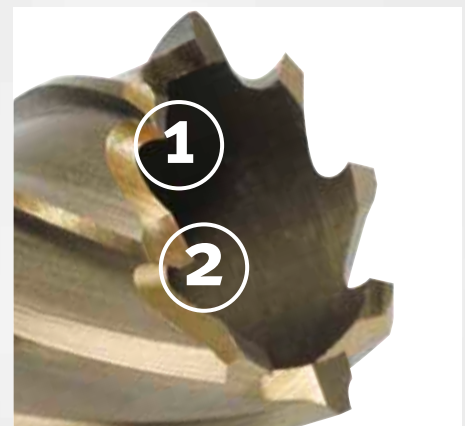
Heavy duty serration with pre- (1) and post-cutter (2)
