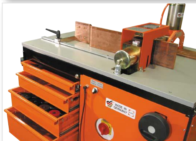
There are 4 tool drawers with compartments for hole punches and dies in the cart.
