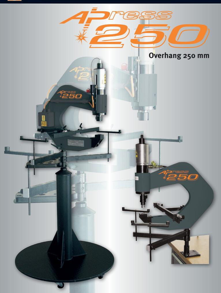
For rapid punching-out of circular, square, rectangular or special forms without pre-drilling in control cabinet doors, terminal boxes, cable ducts, housings, cable management panels etc. right up to margins. Simple tool change carried out in seconds.
