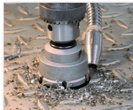
Drilling in checker sheet
