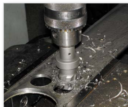
Drilling flat steels
